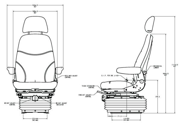
Large mechanical suspension with 3 position height adjustment & double acting Duo® damper.
