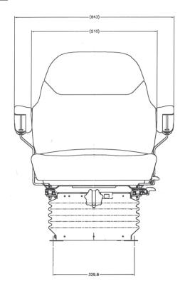
Large mechanical suspension with 3 position height adjustment & double acting Duo® damper
