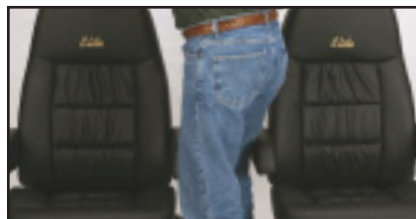
Positioned up or down, the armrests of most seats make moving from the front to the back of the cab difficult.
